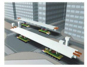
Batch erection of girders in the center span by large transport vehicles
