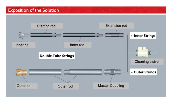
The dedicated drilling tools are basically composed of the inner and outer strings, and drilling is done in the state of the dual tube strings.
