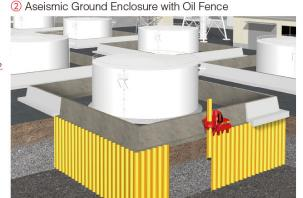
Enclosing sheet piles are repositioned outside the oil fence and connected each other to reinforce against subsidence or turnover caused by forces of earthquake or tsunami.
