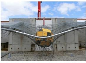
[Full-scale Test: Shallow landslide 100 tons]
