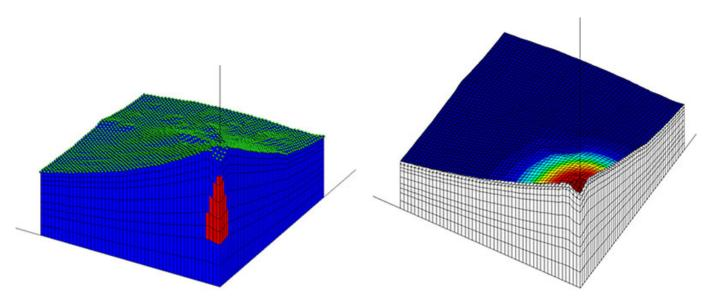
left side: Fig. 1 Mountain and shrinkage area (indicated by red). right side: Fig. 2 Ground surface displacement contour obtained by inverse analysis.
