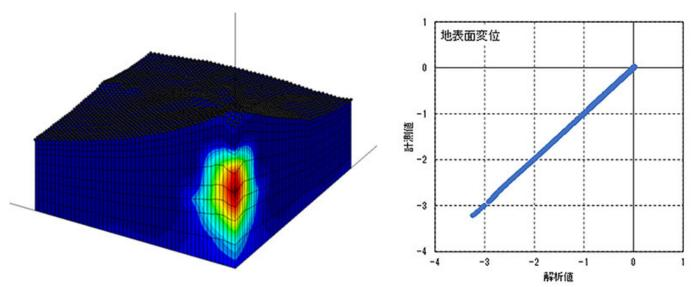
left side: Fig. 3 Shrinkage contour obtained by inverse analysis. right side: Fig. 4 Correlation between measurements and results obtained by inverse analysis.
