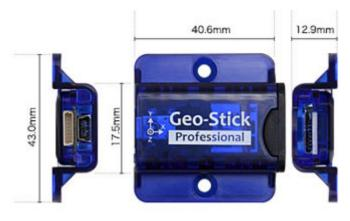
Acceleration data measured by Geo-Stick are sent to the cloud, and then the maximum acceleration and maximum interlaminar deformation angle for each floor are calculated. With these values the degree of damage is determined in comparison with threshold values.
