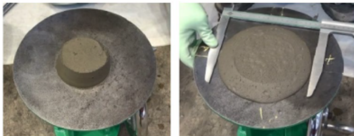
Flow test Mortar with excellent plasticity
