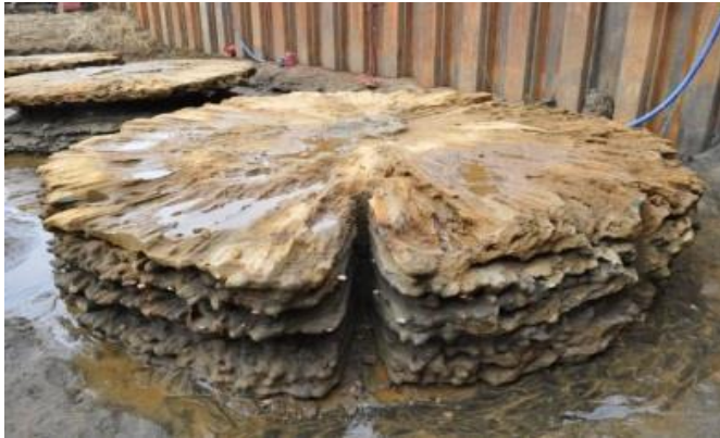
Figure 14. Excavated column and erosion around measuring pipes (case C)
