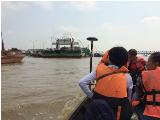
Bathymetric Survey at Lower Bago river CS-6 Survey by RTK combine with Echo sounder
