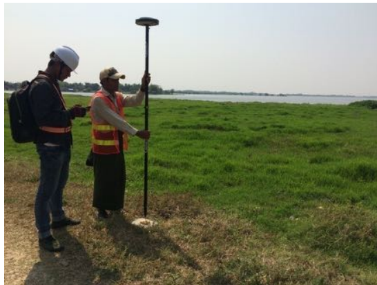
RTK survey on base point checking
