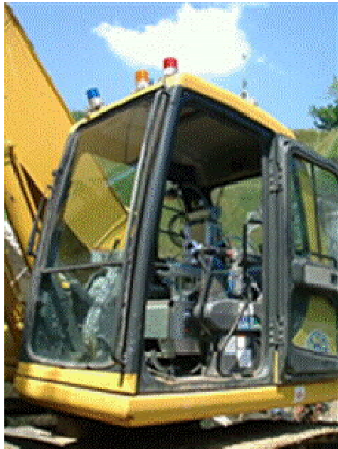
Tele-operated robot for backhoe shovels (Robo Q)
